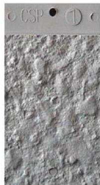
CSP-7: Heavy Abrasive Blast
