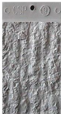
CSP-9: Heavy Scarification
